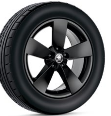
RATIKON Tyre: 215/55 R17 (4×2) 225/55 R17 (4×4) Rim: 7.0J × 17" ET 45 Colour: black metallic design, brushed Code: 57A 071 497D FL8
