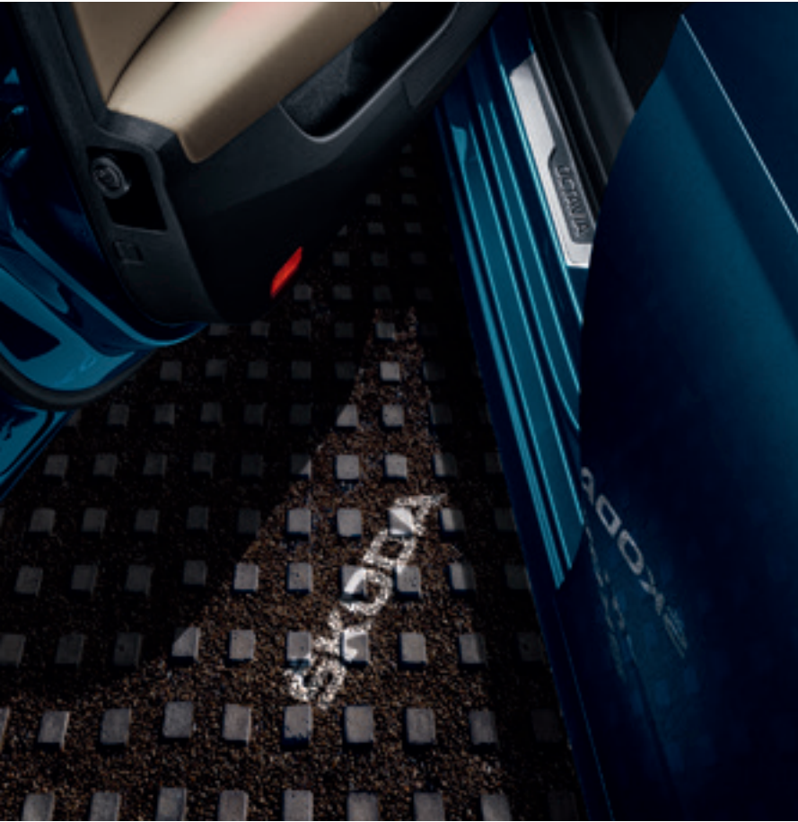
WELCOME LOGO The LEDs located on the underside of the front doors, creating the ŠKODA inscription, illuminate the entry area.
