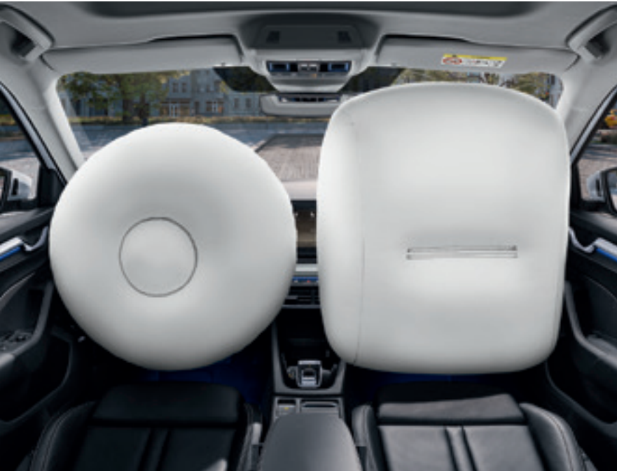
FRONT DRIVER AND PASSENGER AIRBAGS While the driver airbag is enclosed in the steering wheel, the passenger airbag is located in the dashboard. If needed, this can be deactivated when a child seat is installed on the front seat.
