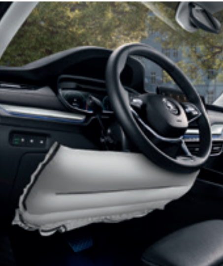
KNEE AIRBAG This airbag, which is located under the steering wheel column, protects the driver's knees and shins.
