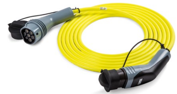
Cable for public charging available as a spare part The MODE 3 cable is for public charging networks. This product is for charging stations that don't have a charging cable or are equipped with an unsuitable one. The cable length is 6m.
