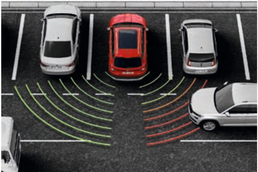
REAR TRAFFIC ALERT This assistant, which comes as part of the Blind Spot Detect system and uses the same radar sensors, helps you reverse safely from a parking space during poor visibility. It can even engage the brakes automatically if it detects imminent danger.
