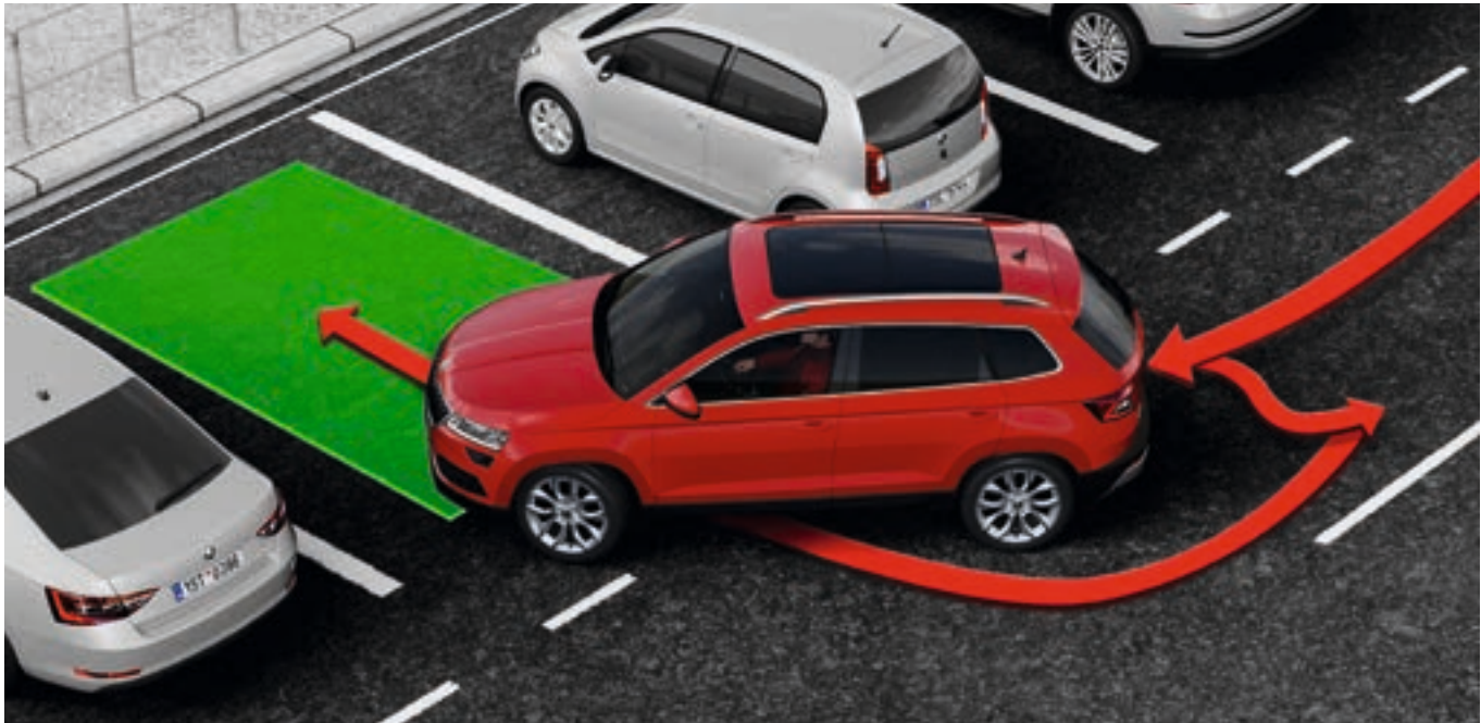
PARK ASSIST Minimise the hassle of parking in tight spots with Park Assist. It automatically selects an appropriate parking place in a row of parallel or perpendicularly parked vehicles.
