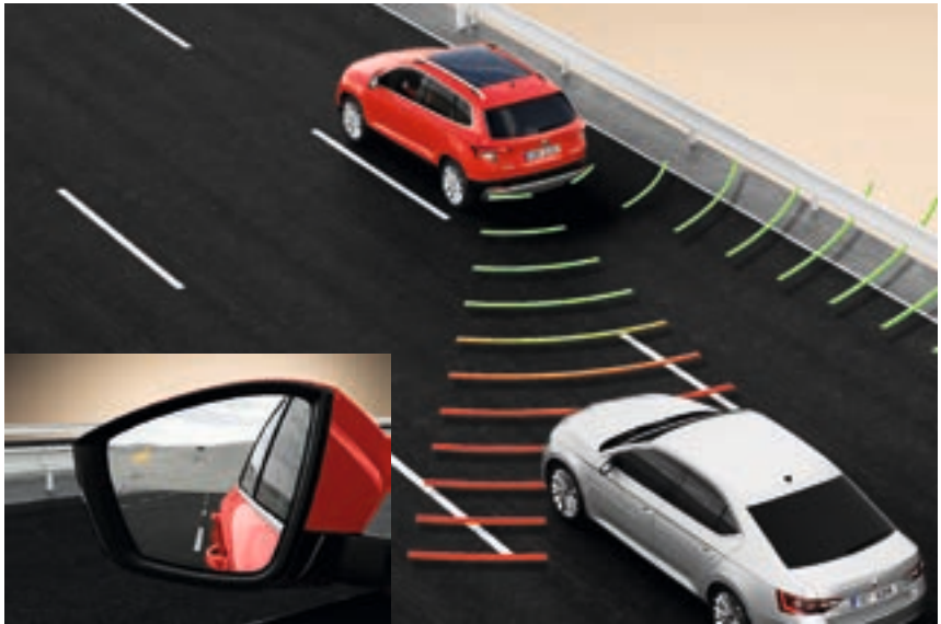
BLIND SPOT DETECT Using radar sensors in the rear bumper, Blind Spot Detect monitors the hidden areas behind and beside the car. Based on the distance and speed of the surrounding vehicles, it decides whether or not it should warn the driver.
