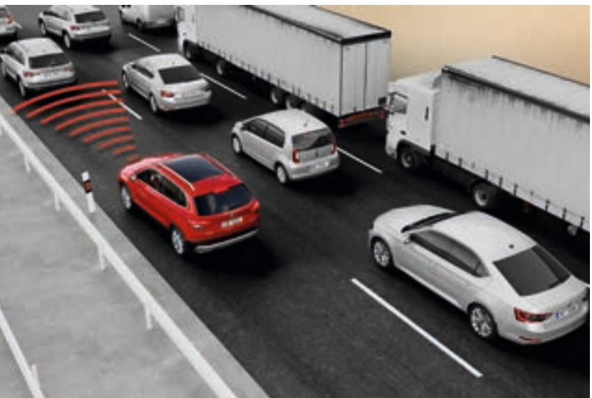
TRAFFIC JAM ASSIST The function is designed to facilitate the driving of DSG-fitted vehicles in traffic jams. By controlling the engine, brakes and steering, it makes the vehicle pull away, brake and turn to copy the movement of the surrounding vehicles (at speeds of up to 60 km/h).
