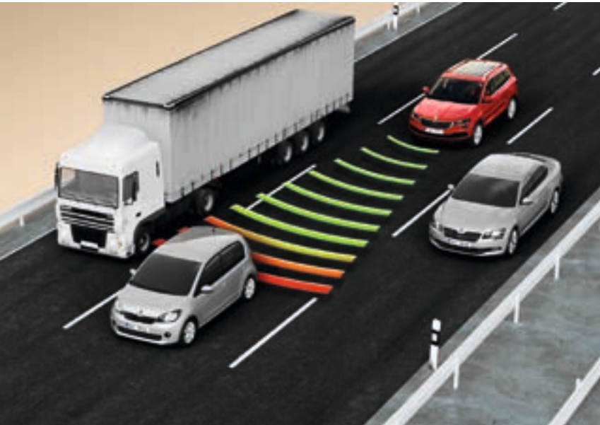
ADAPTIVE CRUISE CONTROL Using a radar device in the front grille, this assistant system maintains a safe distance from vehicles in front of you, in addition to its basic cruise control function.
