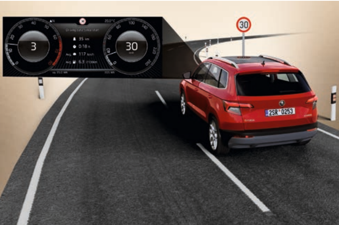
TRAVEL ASSIST This helper uses co-operation between the multifunction camera and the navigation system to recognise and display certain traffic signs on the navigation and Maxi DOT/Digital Instrument Panel screens.
