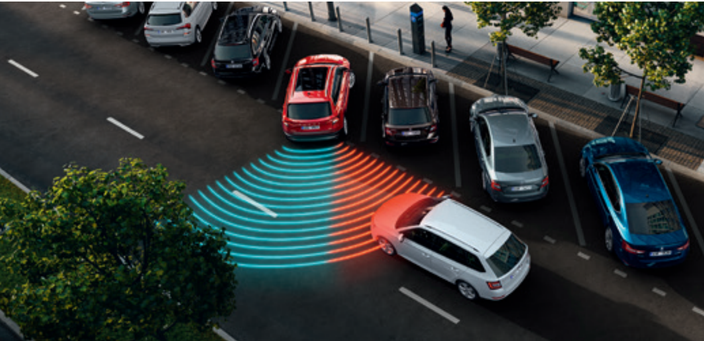
REAR TRAFFIC ALERT The system warns the driver of rear traffic as they pull away from a row of perpendicularly parked vehicles (visually on the infotainment display/ onboard computer display or acoustically), or, if the case so requires, intervenes proactively, i.e., stops the car.
