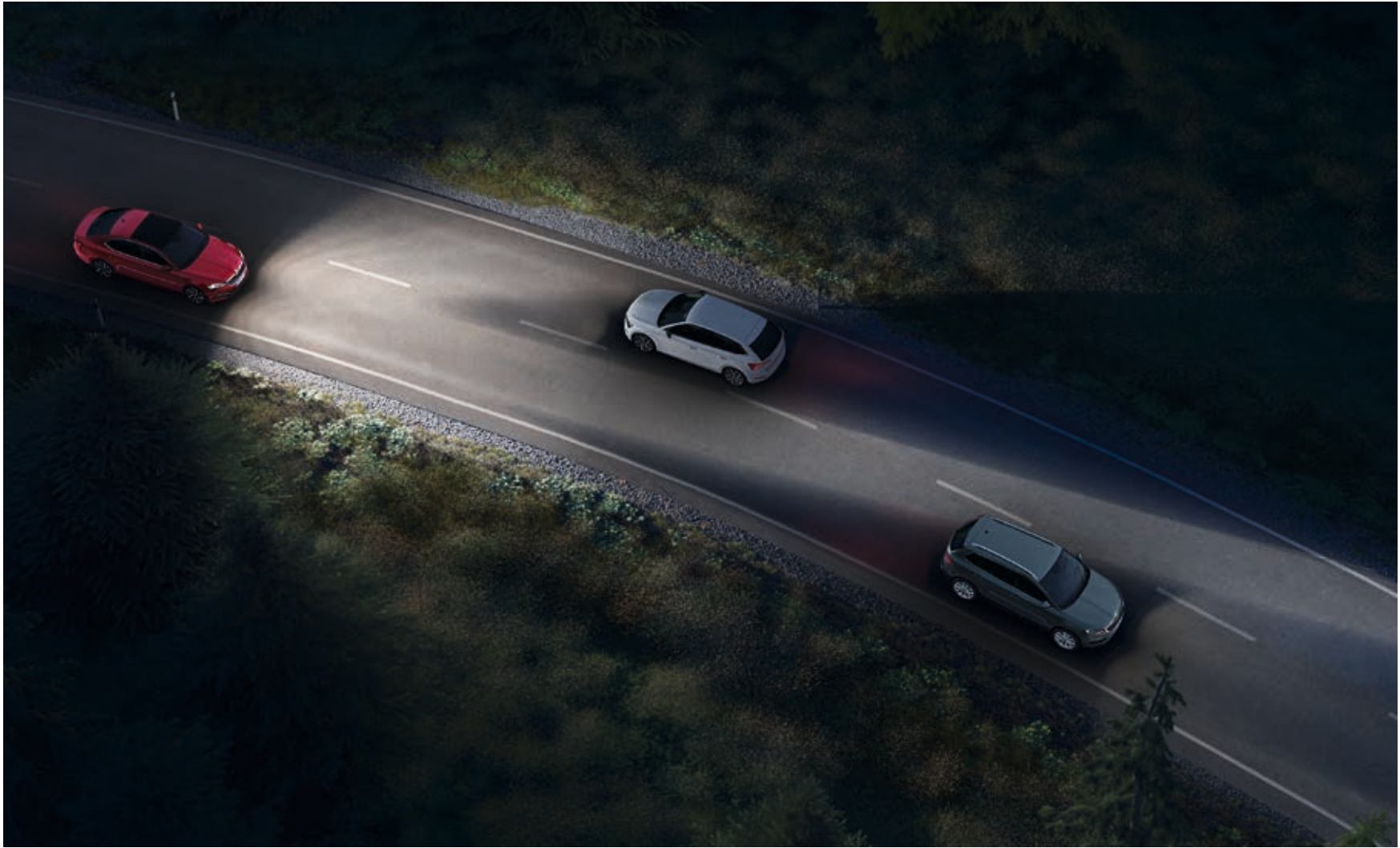
MATRIX BEAM FUNCTION The full LED Matrix headlights feature matrix beam function. This allows you to use the high beams continuously, without blinding other drivers. Using a windscreen camera, the matrix beam function responds to the traffic situation and turns off only some segments of the light. Other segments are turned on and illuminate the road. The matrix beam function also uses information from the navigation system. Thanks to it, the high beams will only turn on when you are out of a built-up area.
