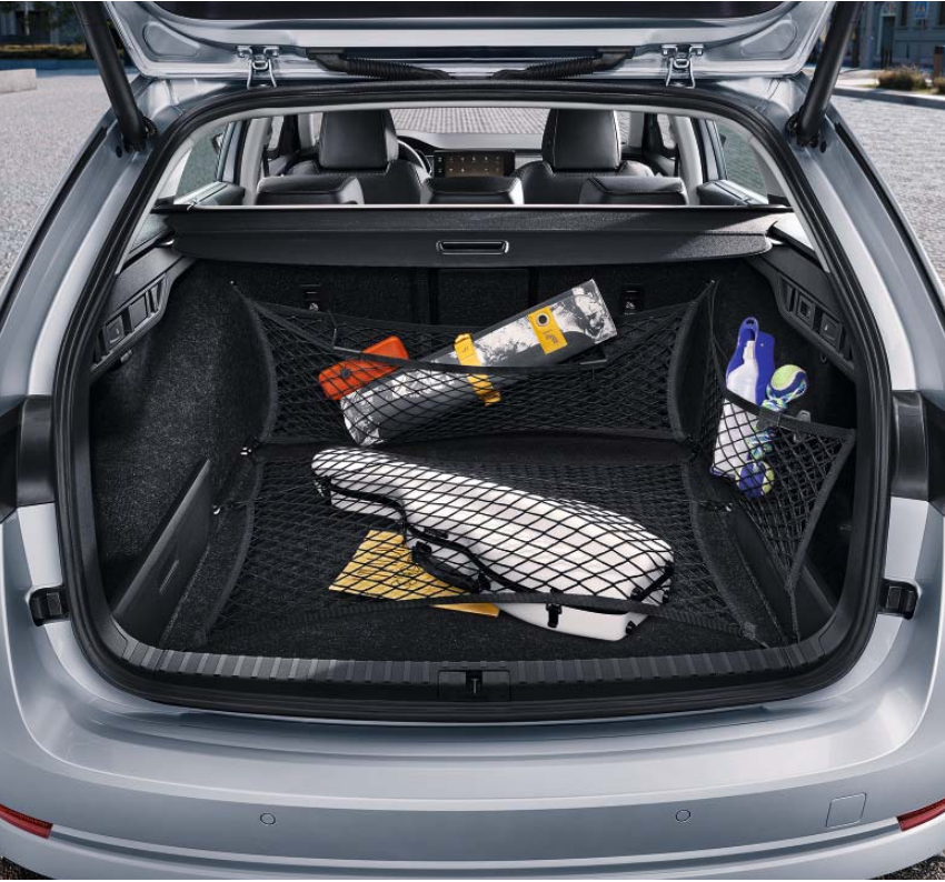
NET PROGRAMME One horizontal and two vertical nets increase the flexibility of the luggage space while firmly securing objects.
