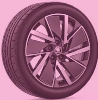
18" VEGA black metallic brushed alloy wheels 7.5J x 18" ET48 for 225/45 R18 tyre
