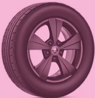
16" VELORUM black metallic alloy wheels 6.5J x 16" ET46 for 205/60 R16 tyre
