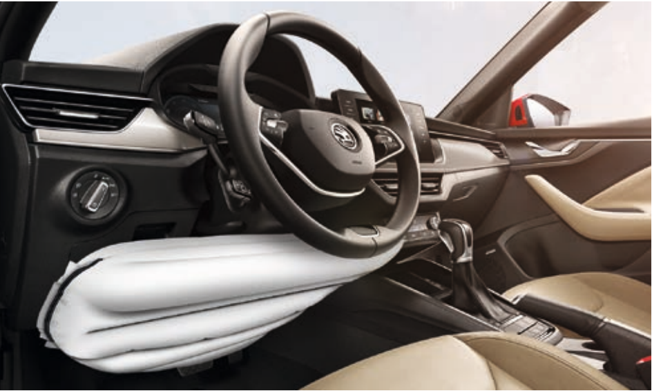
KNEE AIRBAG This airbag, which is located under the steering wheel column, protects the driver's knees and shins.
