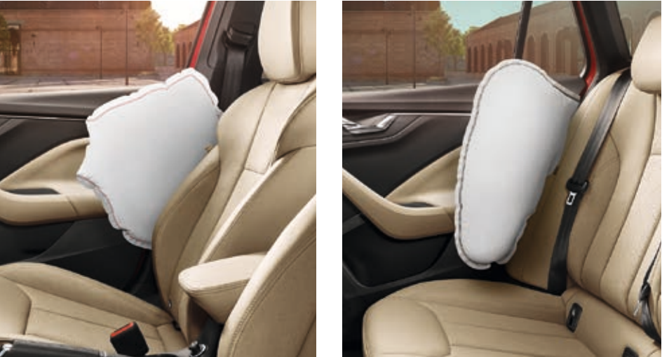
FRONT AND REAR SIDE AIRBAGS These four airbags protect the pelvis and chest of the driver and other passengers in the event of a side collision.
