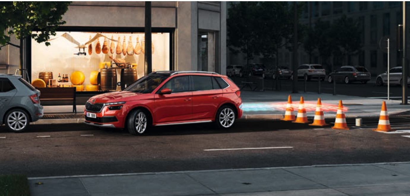
MANOEUVRE ASSIST Using the sensors of the Park Assist, this system offers protection from obstacles within driving distance of the car (at speeds of up to 8 km/h). If an obstacle is detected, based on the distance from the obstacle and the car's speed, the system engages the emergency braking.
