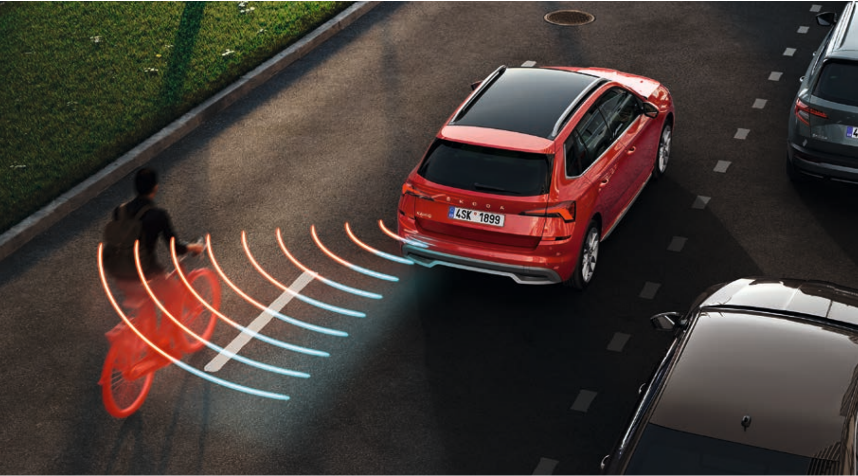
SIDE ASSIST Using radar sensors in the rear bumper, Side Assist which can detect other vehicles and even less detectable objects like cyclists up to 70 m away, monitors the areas behind and beside your car. Based on the distance and speed of the surrounding vehicles, it decides whether or not it should warn the driver.
