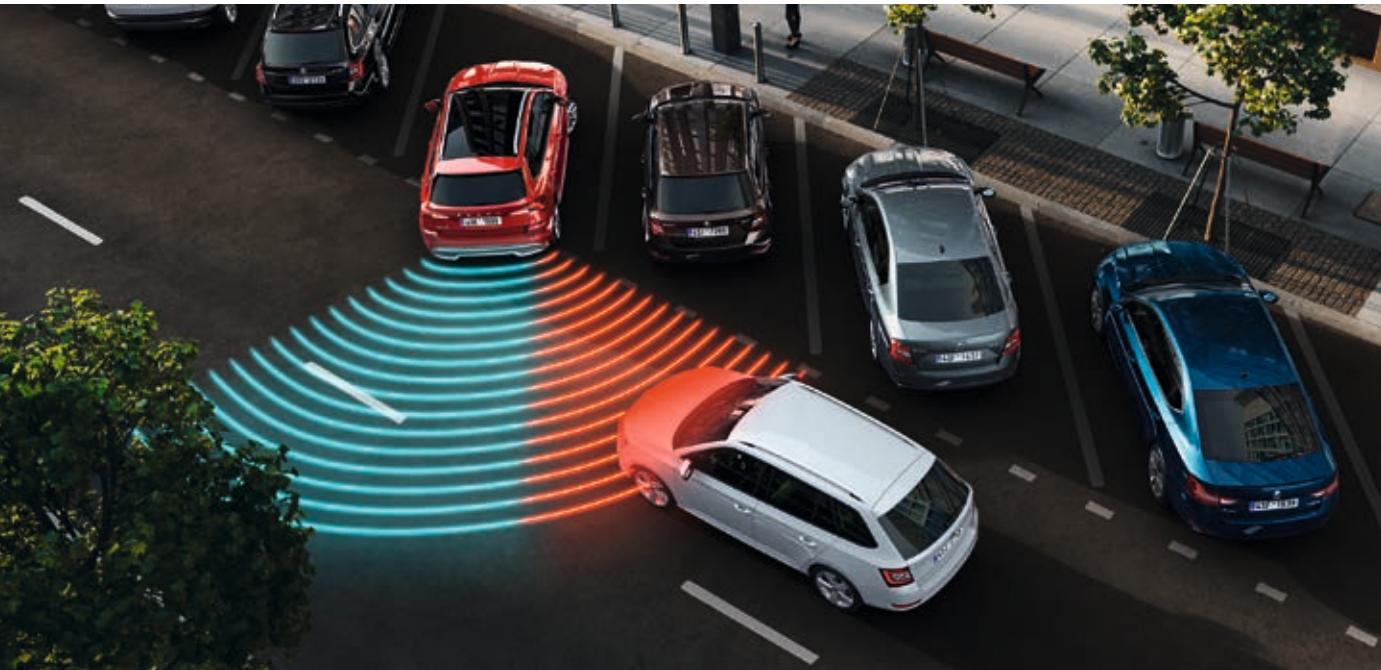
REAR TRAFFIC ALERT This assistant, which comes as part of the Side Assist system, helps you reverse safely from a parking space during poor visibility. It can even engage the brakes automatically if it detects imminent danger.
