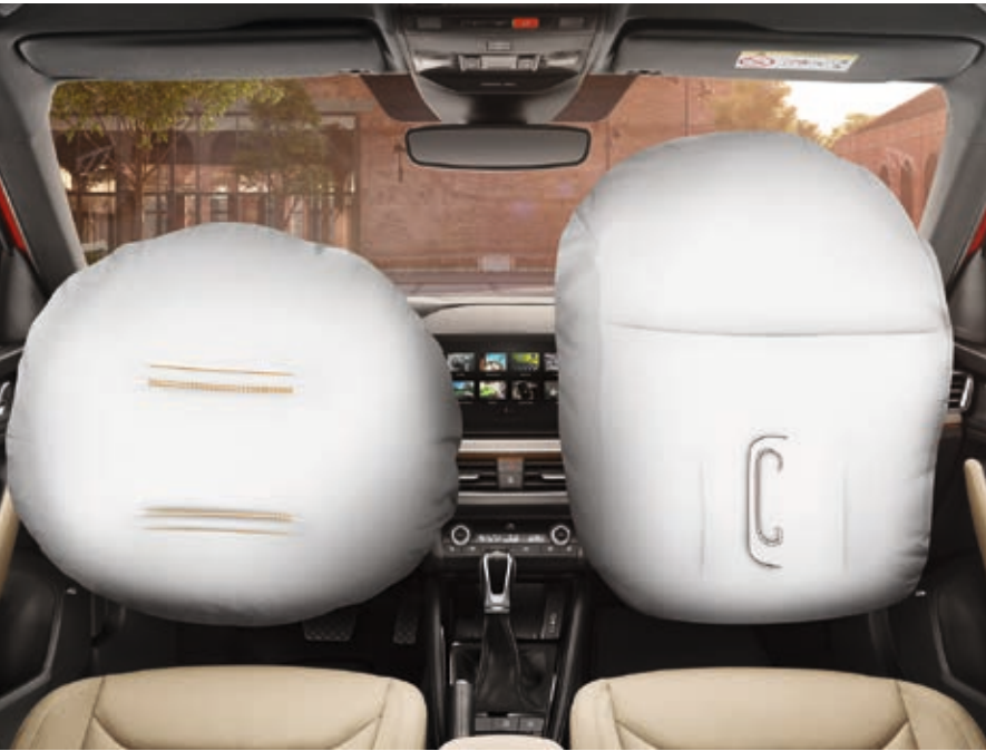
FRONT AIRBAGS While the driver airbag is enclosed in the steering wheel, the passenger airbag is located in the dashboard. If needed, this can be deactivated when a child seat is installed on the front seat.
